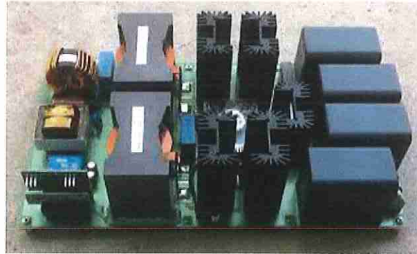
Figure 6: Main Power Board with MCU and Auxiliary Modules
