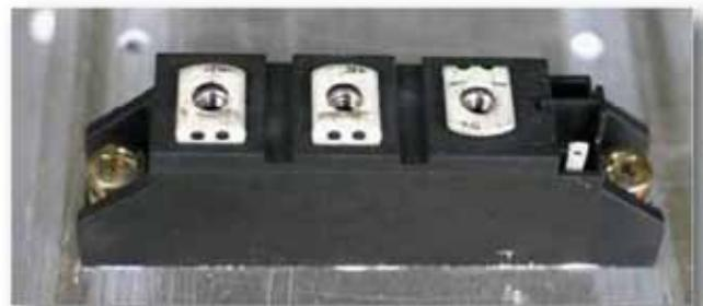
Fig. 3: Mounted device with a thickness of  $60 \mu\text{m}$  thermal grease. That is a strong hint for too much thermal grease.
